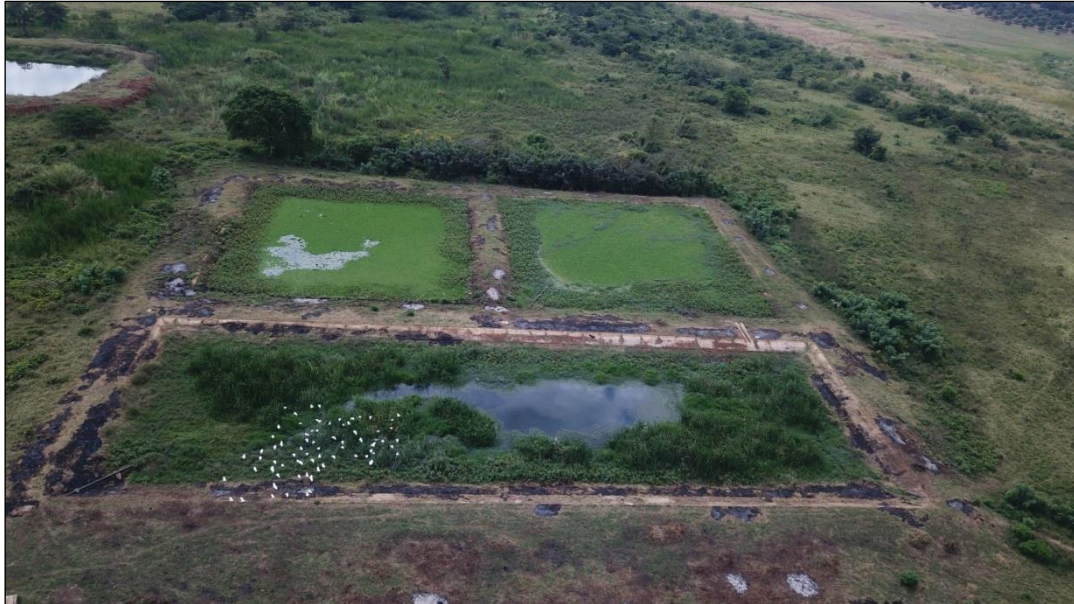
Plate 18: EMC Waste stabilisation ponds (One facultative pond and two parallel maturation ponds) (Photo taken in August 2023)
